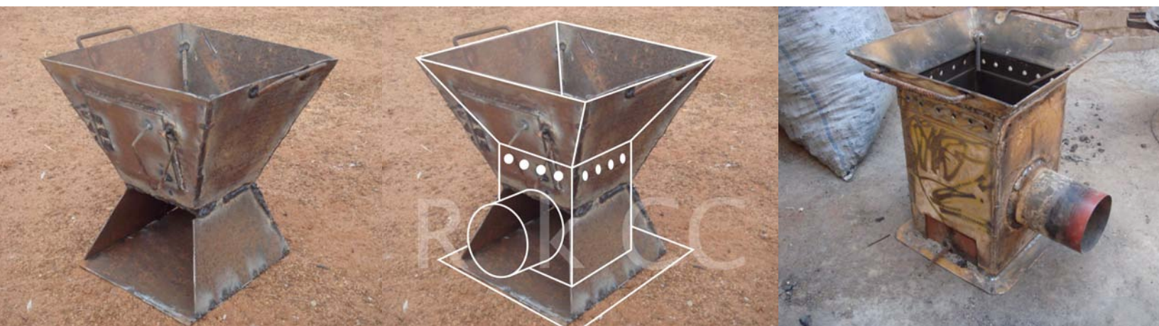
Figure 14: Chad Prototype; an existing stove; a sketch over the photo to suggest the construction adaptation (part of the Creative Commons initiative); the prototype of an adapted stove (photo: Mark Heath, February, 2009)
