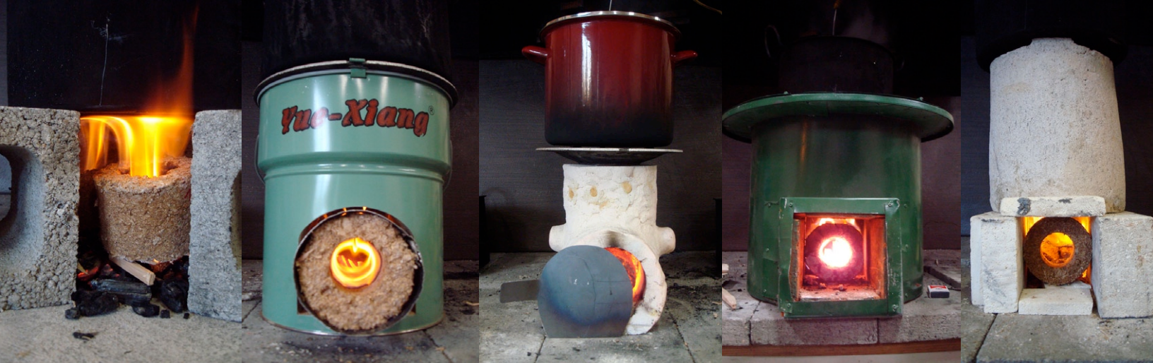
Figure 12: tested stoves: '3-stone' fire, Aprovecho 'China' stove, Holey Rocket, Larry Winiarski rocket stove (Nicaragua), an improvised very high combustion chamber
