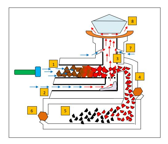
The diagram above illustrates the flow of air, hot gases and char in the stove unit.
