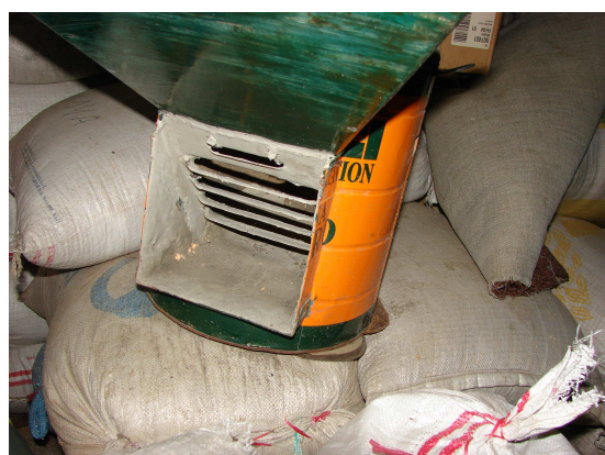
The traditional model of the rice hull stove with step ladder grate. (by the Author).
